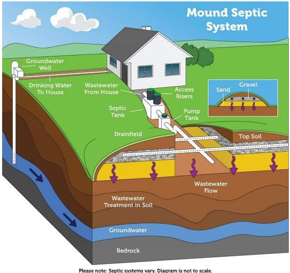
Figure 1.6 - Diagram of a Mound System (USEPA, 2018)
