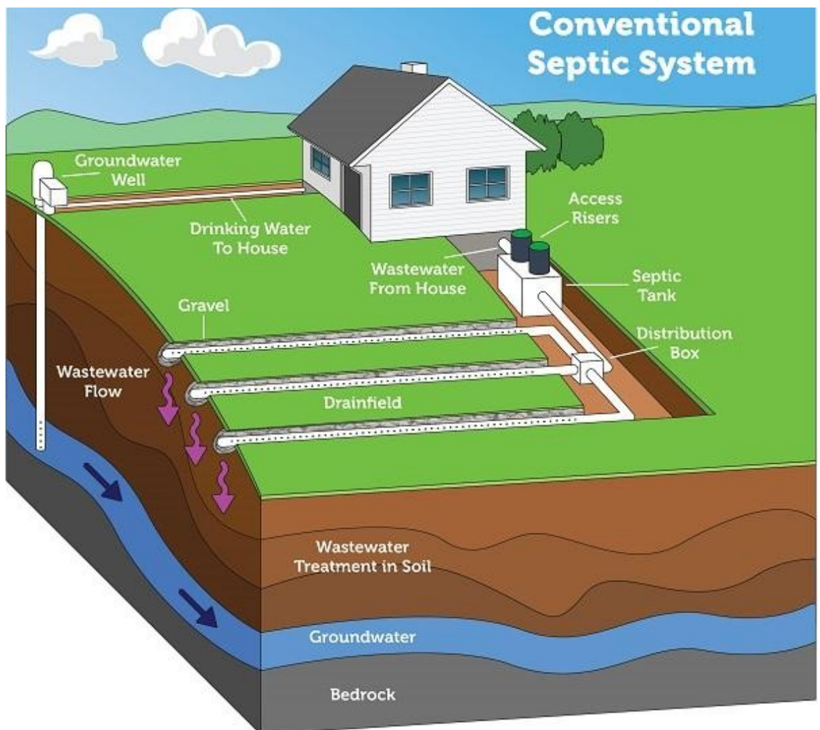
Figure 1.5 - Diagram of a Conventional Septic System (USEPA, 2018)
