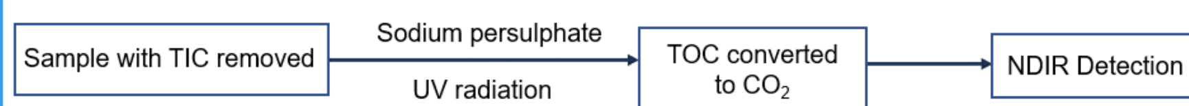
Figure 1. TOC analyser principle of operation schematic.
