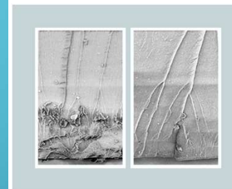
Fig. 7 SEM at x1000 magnification of water washable resin after a 24hr thermal cure at 60°C with no immersion (left) and water immersion (right)
