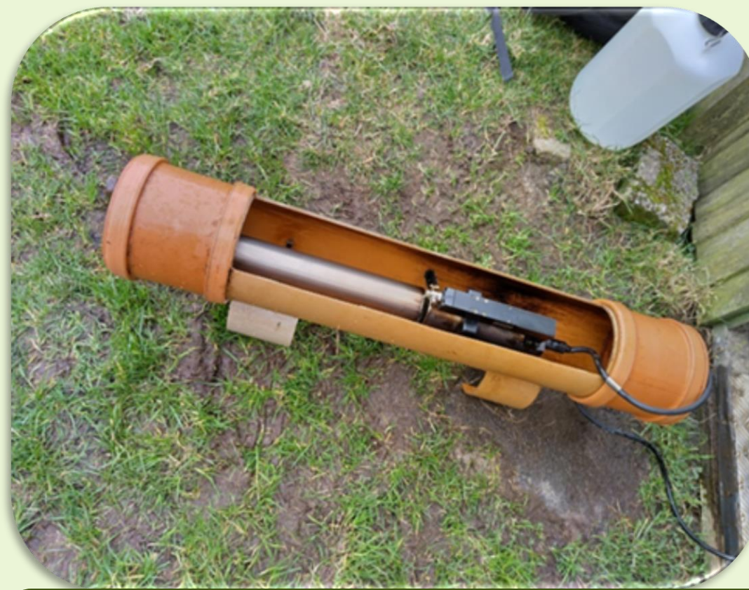
Figure 1. The SUNAV2 inside a 10-litre chamber in which it measures the \text{NO}_3 concentrations of the water flowing in
