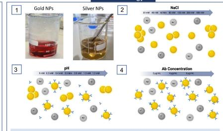
(1) Synthesis of stable, monodispersed gold (Au) and silver (Ag) nanoparticles. (2) Analysis of nanoparticle aggregation behaviour in varying alkaline environments. (3) Use of K<sub>2</sub>CO<sub>3</sub> to modify the colloidal solution pH during antibody attachment to the nanoparticles. (4) Stability study of nanoparticles at varying antibody concentrations under controlled pH and NaCl conditions.
