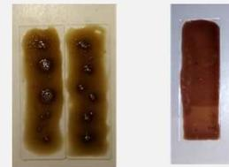
Figure 4 - Drop cast slides (left) vs Spincoated slides (right)
